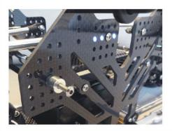
The upper links can be moved by the same number of holes to keep the angle of the gearbox the same, these holes are also 1/4" apart.
