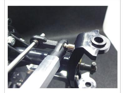
The top link mounts attach to the gearboxes as shown, 1x 6mm spacer at the rear and the 3 x cut washers at the front.
