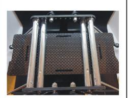
The brass weights can be added to the chassis to aid stability, between 1 and 4 can be used.
