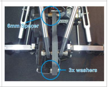
The wheelbase can be adjusted between 12" and 13.5" by changing where the lower arms attach to the chassis.
