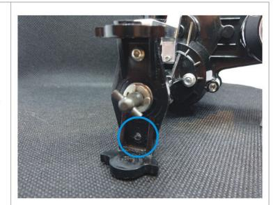
Put the 4mm spacer over the screw first, then the lower link. Slide the rod end over the sway bar wire before attaching it.
